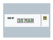
One camera could inspect a date code and a 2D code, both in the field of view but each with their own region of interest. This is a very cost effective method for checking both date code and artwork.
