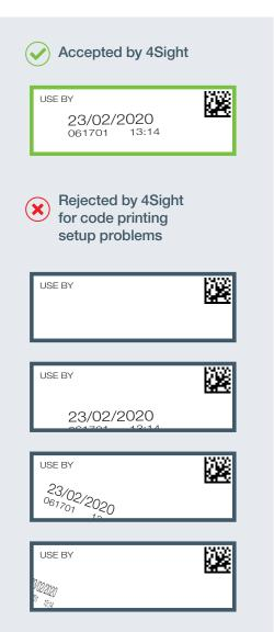
Although 4Sight's Inspection Depth does extend to OCR, it is not recommended for inline print inspection applications. This is due to the reliability challenges of using OCR-based algorithms. By using Print Box Detection, 4Sight delivers exceptionally reliable results at a fraction of the processing time.
