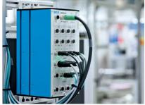
Using the SICK SIM4000, 4 cameras can carry out 4 different inspections.
