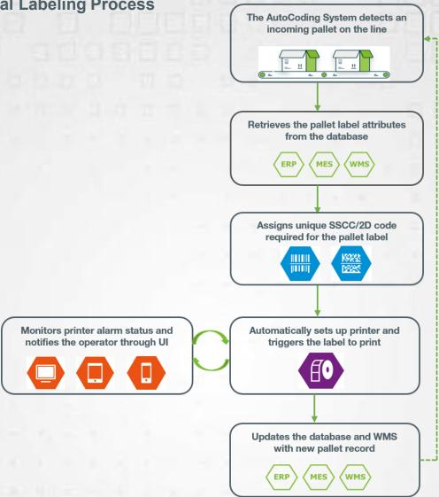
Once an incoming pallet is received, the AutoCoding system detects the pallet through I/O communication with an existing PLC or by triggering a scan of the cases of product on the pallet.
