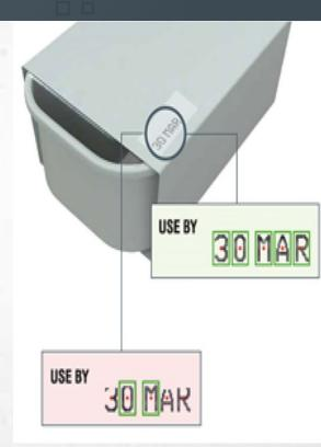
However, more typically you would stop the line if you have a number of instances of poor codes in a row, for example. This eliminates the nuisance line stop from just one poor code which can be very helpful. Importantly, the user can choose how to set the system up and what the definition of bad and poor code is for them, as well as what to do when one is detected.
